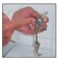
Remain body of the assembly kit is fixed to washbasin assembly bolt, with the help of nuts, as shown on the above.
